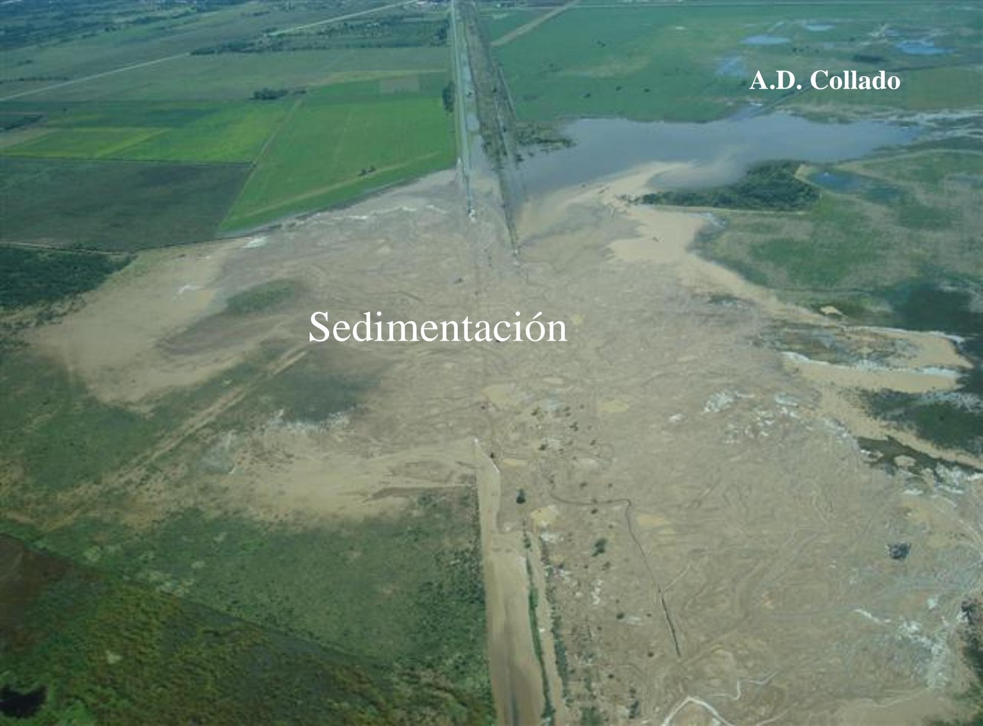
An aerial photograph showing a long dam structure extending from the top center towards the bottom center. The reservoir behind the dam is filled with a thick layer of brown sediment, which has accumulated in a large, irregular shape. The surrounding landscape consists of green agricultural fields and some water bodies. The text 'Sedimentación' is overlaid on the sediment area, and 'A.D. Collado' is in the top right corner.
